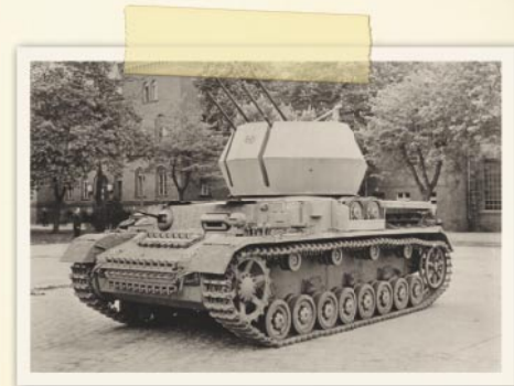
Watch out for this one: a Panzer IV tank chassis with quadruple 20 mm flak guns.
